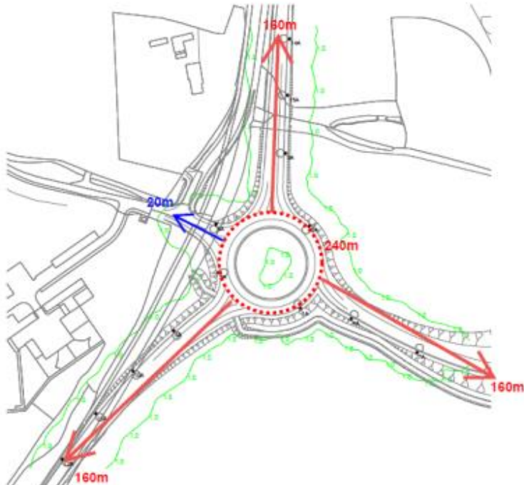
Figure 2 – Distances used in lighting assessment
